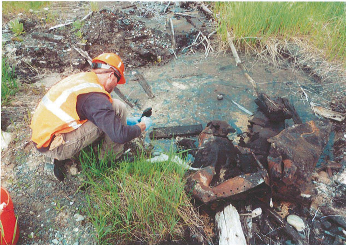
Photo 4: 6/15/11 - BNSF contractor collecting sludge sample from a sludge pit on the eastern portion of the KRY Site.
