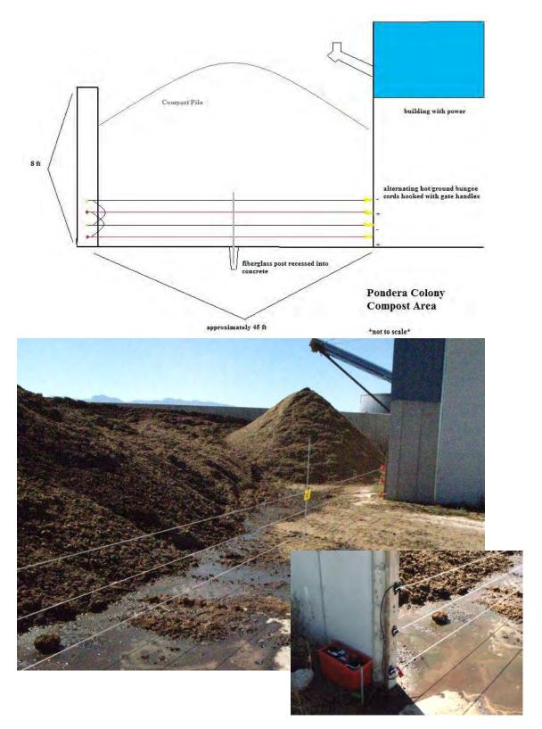
Figure 2. Design and installation of a portable 12v-converted to AC powered electric fence system to deter grizzly bear access into the Pondera Colony livestock carcass compost facility, 9/20/2013.
