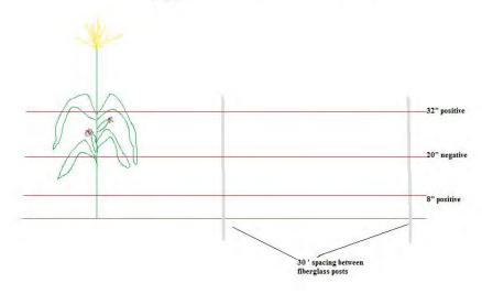
Figure 1. Portable/temporary electric fence design to deter grizzly bear access to Pondera Colony silage cornfields.
